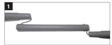
Handle Assembly – insert the 3 handle pieces into each other – be sure to push the wire into the handle slots. Pull any excess cord through from plug. Use the screws provided to complete the assembly.
